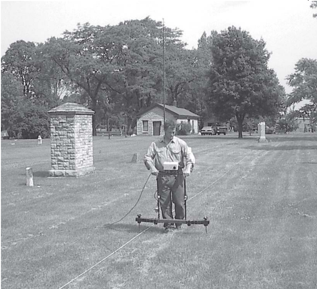
The author conducted an electrical-resistance survey at Layman's Cemetery. The probes at the bottom of the frame measure the flow of electricity when they are placed in contact with the soil.
